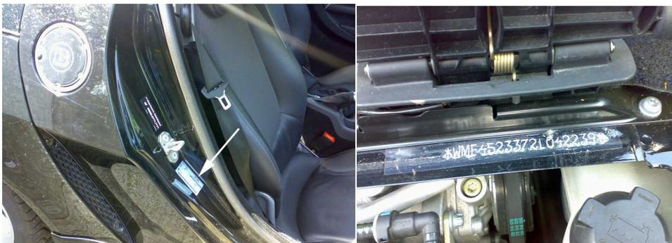
You need to check the chassis number, it is stamped into the edge of the engine bay at the driver's side (RHD) towards the front of the car. It is repeated in the driver's door shut, however, the door shut is only a sticker and may have been removed for cosmetic reasons or worn out! The two numbers should match, and more importantly they need to match the DVLA paperwork for the vehicle. Use the chassis number and registration plate to do an online search of the vehicles history.
