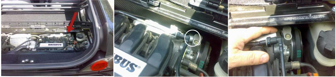
These pictures show a 2005 Brabus Xclusive with a broken pipe after just 12,000 miles. That same car is just about to go in for its FOURTH set of pipes! Look for cracks, not just breaks. Although be warned, they can be so fine you will not see them!
