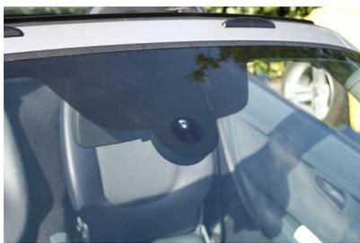
Above: a roadster factory fitted with the automatic wipers. The sensor is easily visible, but it does mean having a different windscreen so it would not be cost effective to fit this to a roadster at a later date.
